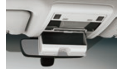
Overhead console gives easy access to interior lights and small-item storage
