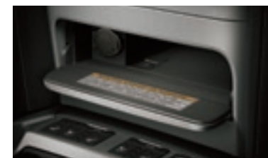
The wireless charger recharges your smartphone battery when you place it on the charger's power pad
