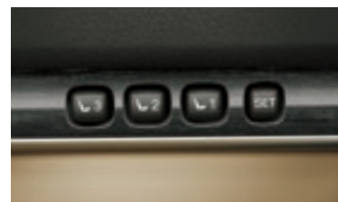
The seat memory function remembers the preferred seat position of three different drivers
