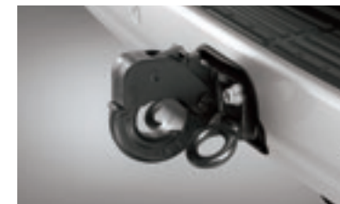
Convenient pintle hook allows towing of trailers and other vehicles
